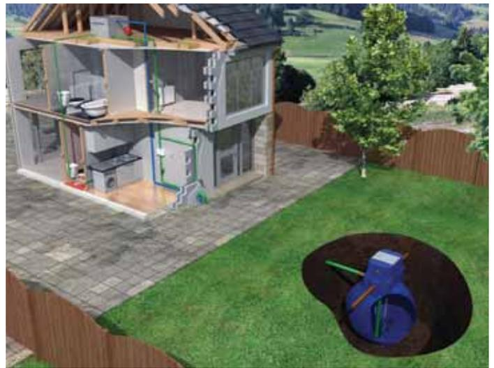
**Splashing out: Modern rainwater harvesting systems are pressurised, meaning they include a pump to get the water from a storage tank directly to the point of use**
